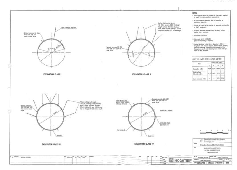
Glendoe Hydro Electric Scheme Headrace TBM excavation Rock Support Methodology 162 – DC – 12 – 20 – 97 – 02 – 00
